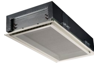
PARASOL is a comfort module for cooling, heating and ventilation via the CONDUCTOR control unit and actuators. Module dimensions 1200x600 or 600x600 mm.
