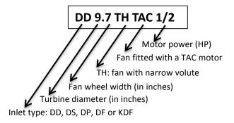
Some fans do, however, have a name for the diameter of the turbine and the width of the wheel in mm.
