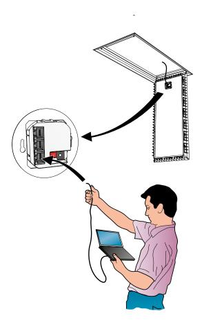
Figure 18. The CABLE CONVERTER USB-RJ12 (RS485) cable can be easily used for connecting a computer to the module for e.g. entering software settings. The cable can be connected either to a socket on the rear of the Sensor module as illustrated, or directly to the controller. How this is done is described in the SWICCT user's manual.
