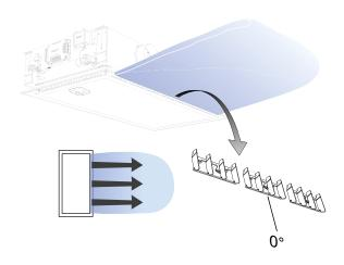
Figure 24. Possible settings for the ADC, Straight airflow setting
