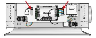
Figure 30. All controll equipment is gathered on the same side to simplify the work during installation and service.
