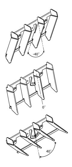
Figure 21. ADC, setting range from -40° to +40° in increments of 10°  $\,$
