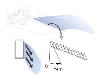
Figure 23. Possible settings for the ADC, X-shape
