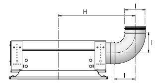
Figure 41. Connection with bend, viewed from end panel Mounted connection piece SYST CA xxx-90
