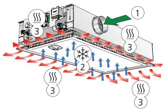
Figure 3. Variant X: Supply air and heating operation with electric heating elements (also includes cooling function)
