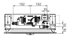
Figure 34. ADAPT Parasol 600, water connections
