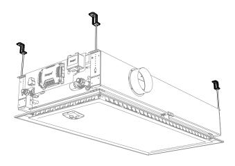
Figure 28. Suspension of a two-module unit
