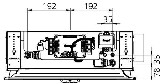
Figure 34. ADAPT Parasol 600, water connections
