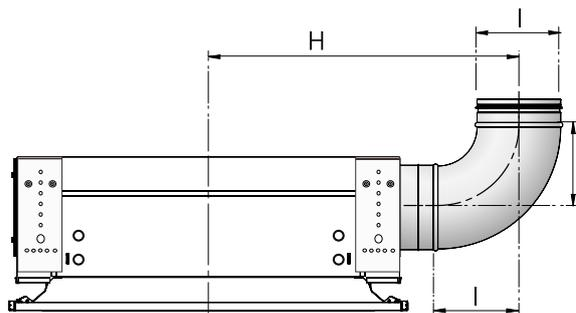
Figure 41. Connection with bend, viewed from end panel
