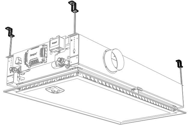
Figure 28. Suspension of a two-module unit
