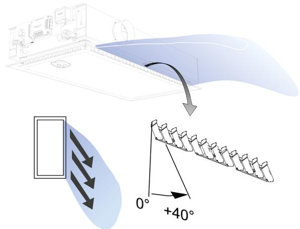
Figure 23. Possible settings for the ADC, X-shape
