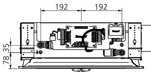
Figure 39. ADAPT Parasol 1200, water connections
