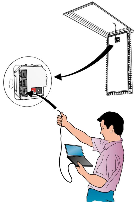
Figure 18. The CABLE CONVERTER USB-RJ12 (RS485) cable can be easily used for connecting a computer to the module for e.g. entering software settings. The cable can be connected either to a socket on the rear of the Sensor module as illustrated, or directly to the controller. How this is done is described in the SWICCT user's manual.
