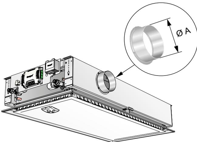
Figure 27. Air connection piece
