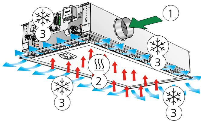
Figure 1. Variant A: Cooling and supply air operation
