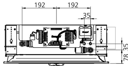
Figure 34. ADAPT Parasol 600, water connections
