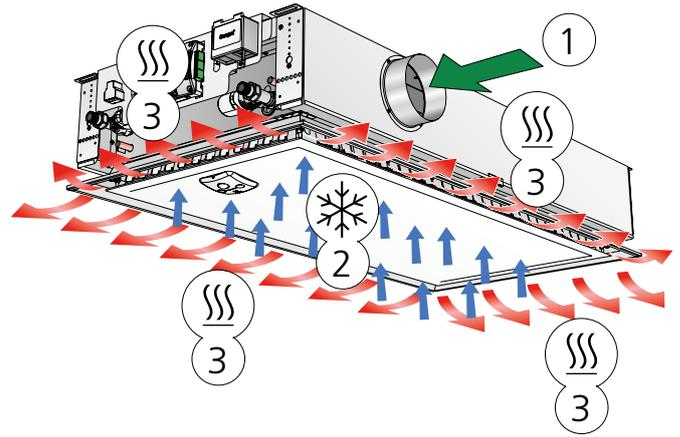
Figure 3. Variant X: Supply air and heating operation with electric heating elements (also includes cooling function)
