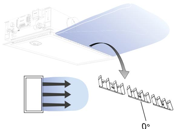
Figure 24. Possible settings for the ADC, Straight airflow setting
