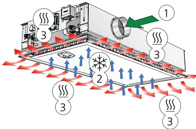
Figure 2. Variant B: Heating and supply air operation (includes also cooling operation)
