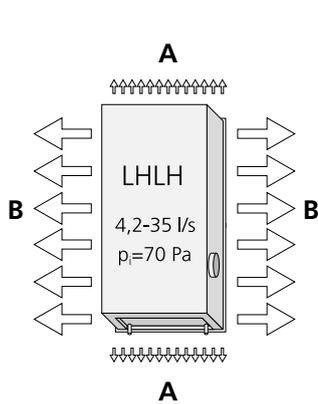
Figure 13. Example 1. A = 2.1 l/s, B = 15.4 l/s
