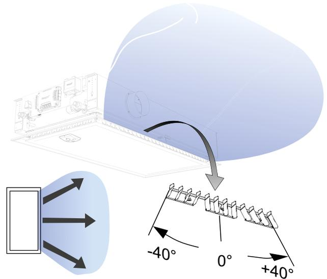
Figure 22. Possible settings for the ADC, Fan shape
