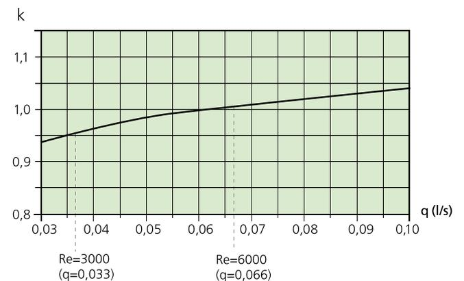
Diagram 4. Pressure drop – Water flow, Cooling
