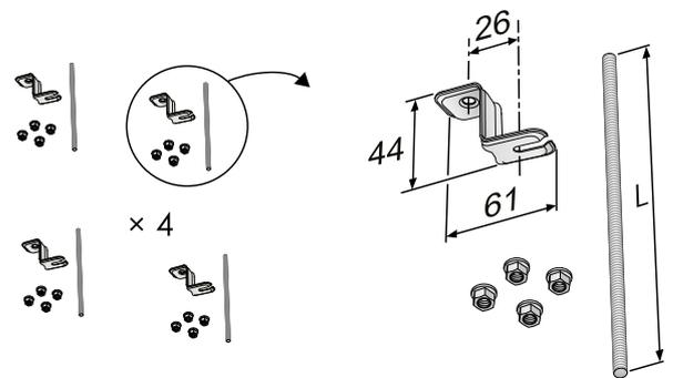
Figure 29. Assembly piece SYST MS M8-1, ceiling mount and threaded rod
