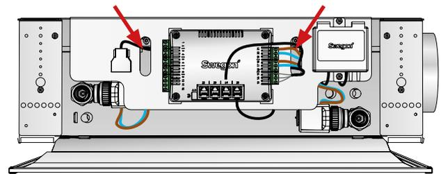
Figure 30. All control equipment is gathered on the same side to simplify the work during installation and service.
