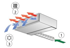
Figure 3. Heating function Paragon Wall 1 = Primary air 2 = Primary air mixed with heated room air
