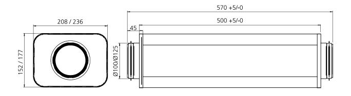
Figure 33. Dimensional drawing sound attenuator CLA Ø 100-500 or Ø125-500. The following components are included in PARAGON T-SAK and PARAGON T-EAK:
