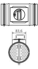
Figure 35. Dimensional drawing commissioning damper. Included in PARAGON T-SAK-CAV and PARAGON T-EAK-CAV
