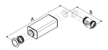
Figure 41. Extract air kit, PARAGON T-EAK-CAV Available for connection sizes 125 and 100. Spiral duct and bends are not included A: Min. length: 770 mm B: Min. length: 360 mm
