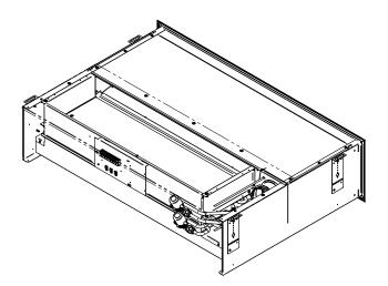
Figure 24 Paragon Wall with factory-fitted LUNA wiring terminals, VEN115 valve and actuator ACTUATORb 24V NC.
