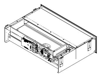
Figure 23. Paragon Wall with factory-fitted Conductor W4.1 controller including RU room unit and 2 pressure sensors as well as CCO valve for cooling and heating.
