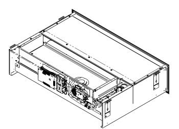
Figure 12. Factory-fitted CONDUCTOR with CCO valve PARAGON WALL B-HC
