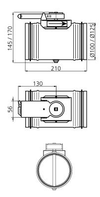
Figure 34. Dimensional drawing motor-driven damper. Included in PARAGON T-SAK-VAV and PARAGON T-EAK-VAV
