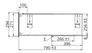
Figure 29. End view E = Condensate drip tray
