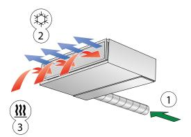
Figure 2. Cooling function Paragon Wall 1 = Primary air 2 = Primary air mixed with chilled room air 3 = Induced room air
