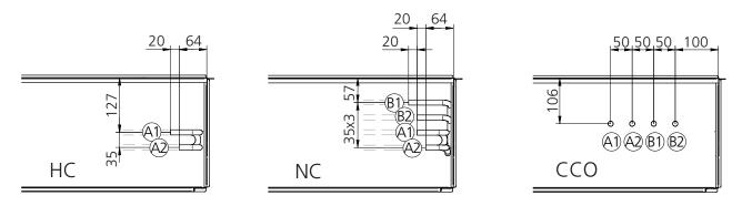
Figure 31. View rear - water connections, A1 = Cooling water, inlet pipe Ø12x1.0 mm (Cu) B1 = Heating water, inlet water Ø12x1.0 (Cu)
