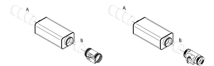
Figure 36. Supply air kit PARAGON T-SAK-VAV-125 Spiral duct not included. Spiral duct A: Min. length: 330mm Spiral duct B: Min. length: 70mm Figure 38. Supply air kit PARAGON T-SAK-CAV-125 Spiral duct not included. Spiral duct A: Min. length: 330mm Spiral duct B: Min. length: 70mm
