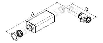
Figure 42. Extract air kit, PARAGON T-EAK-CAV Available for connection sizes 125 and 100. Spiral duct and bends are not included A: Min. length: 770 mm B: Min. length: 360 mm
