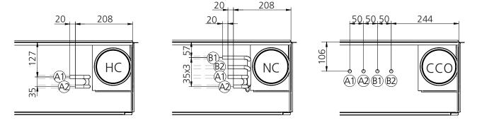
Figure 27. View rear, water connection. A1 = Cooling water, inlet pipe Ø12x1.0 mm (Cu) B1 = Heating water, inlet water Ø12x1.0 (Cu)
