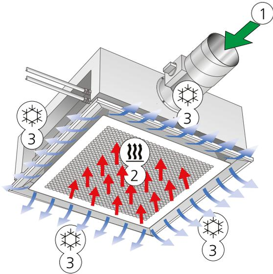
Figure 3. Variant A: Cooling and supply air function
