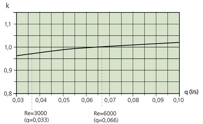
**Diagram 3. Corrected capacity – water flow, PARASOL VAV 1200**
