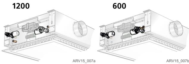
Figure 17. Water connection with factory fitted valves
