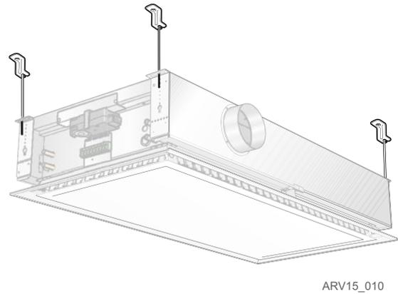
Figure 20. Suspension double-module units
