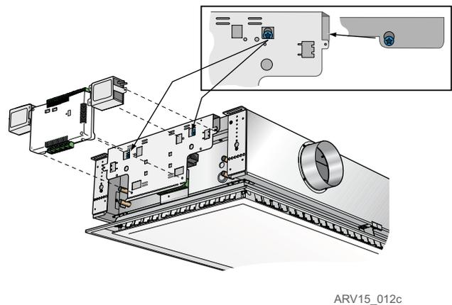
Figure 22. All control equipment is collected on the same short side to facilitate work during installation and service.
