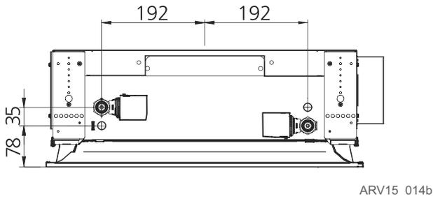
Figure 31. PARASOL VAV 1200, water connection
