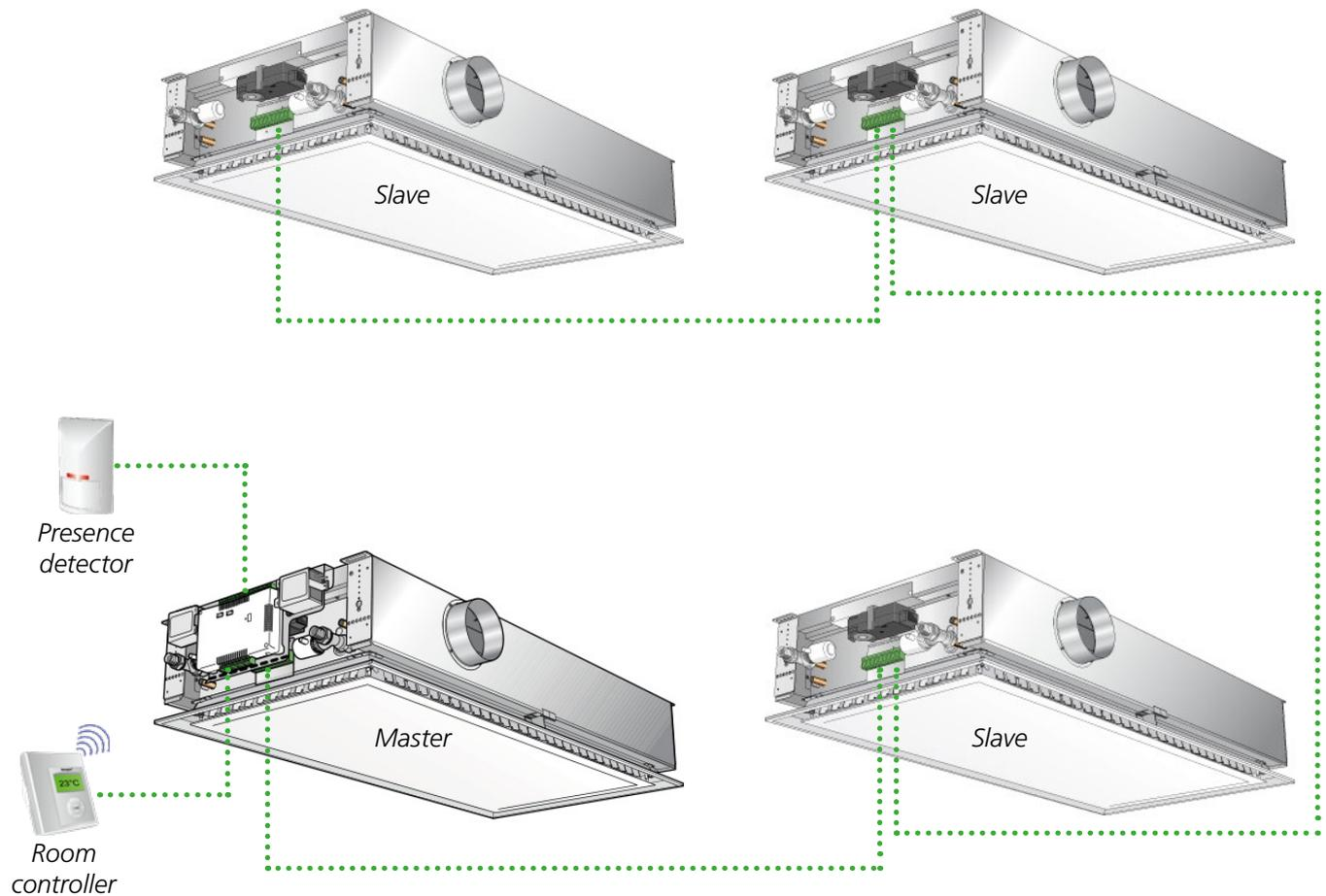
Figure 7. For example on PARASOL VAV Master - Slave connection
