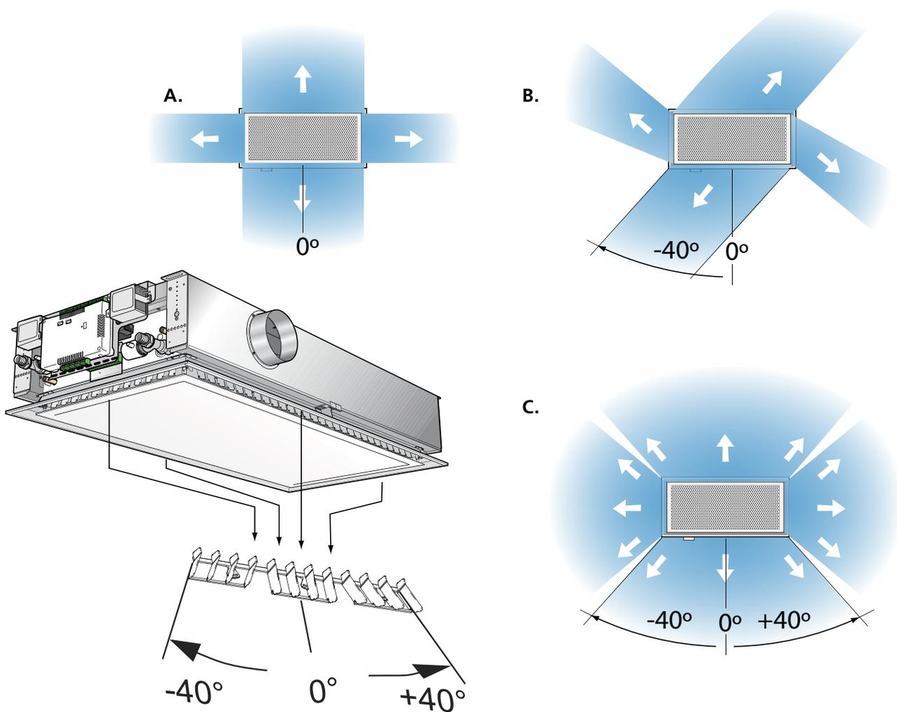
Figure 13. Setting options ADC. Setting range from -40° to +40° in increments of 10°.
