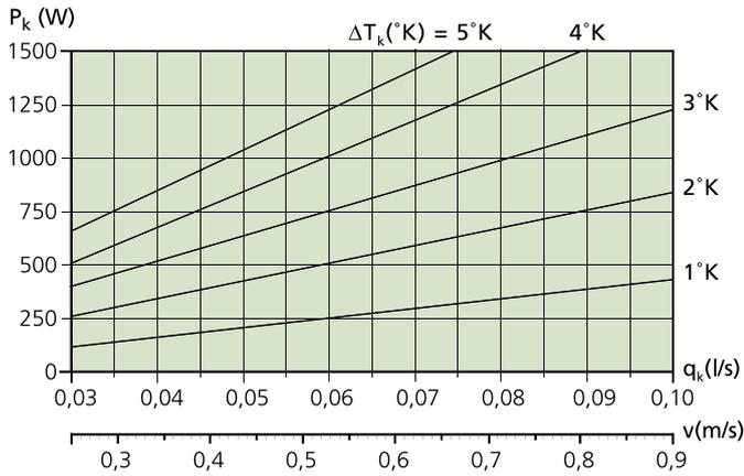
**Diagram 2. Corrected capacity – water flow, PARASOL VAV 600**
