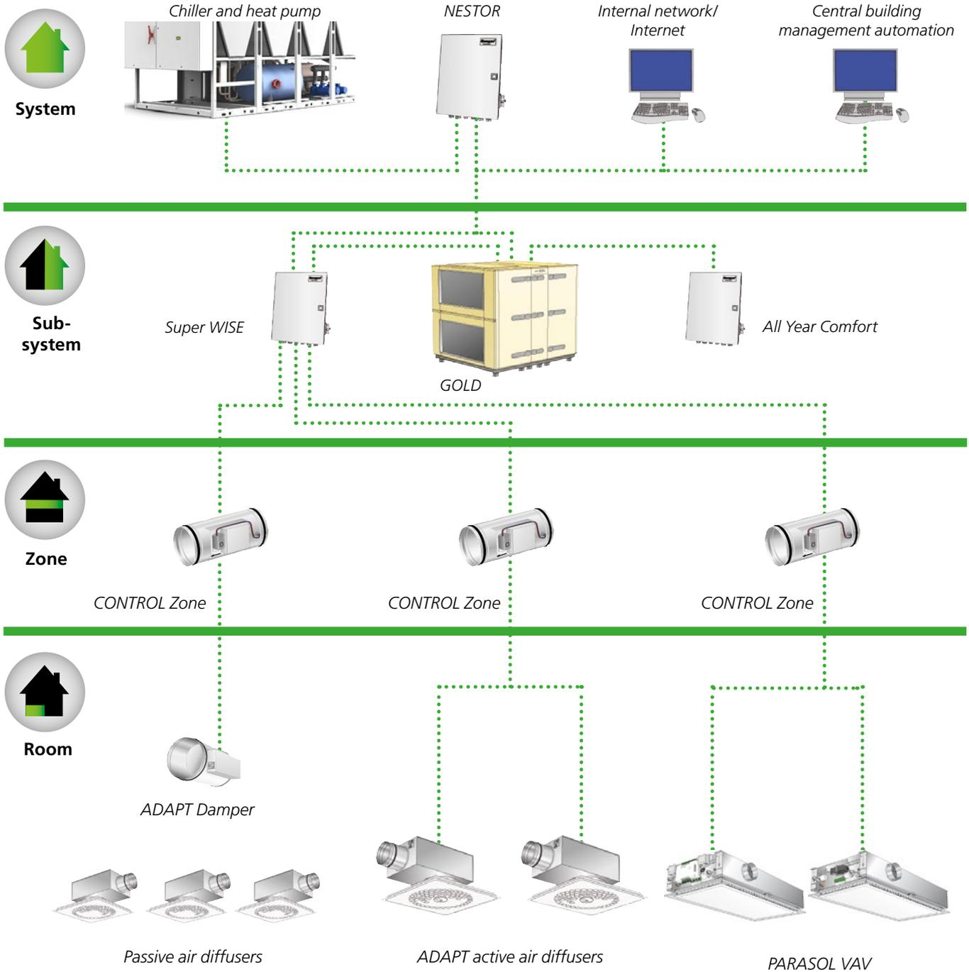
Figure 14. Examples of how the PARASOL VAV can be connected to a WISE system
