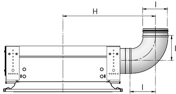
Figure 33. Connection with elbow, short end view
