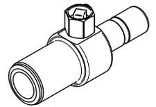
**Connection piece, air – insertion joint, SYST AD1**
