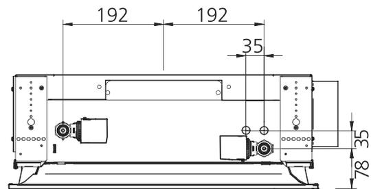
Figure 26. PARASOL VAV 600, water connection
