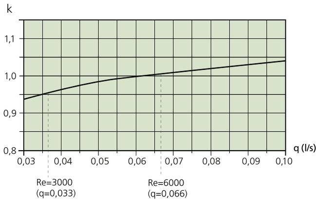
**Diagram 4. Pressure drop – water flow, cooling**
