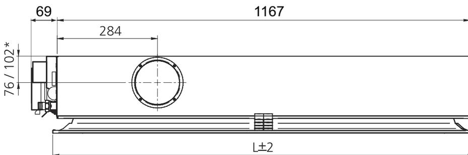
Figure 29. PARASOL VAV 1200, side view
