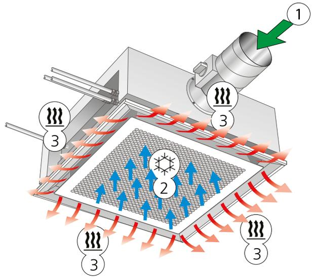
Figure 4. Variant B: Heating and supply air function
