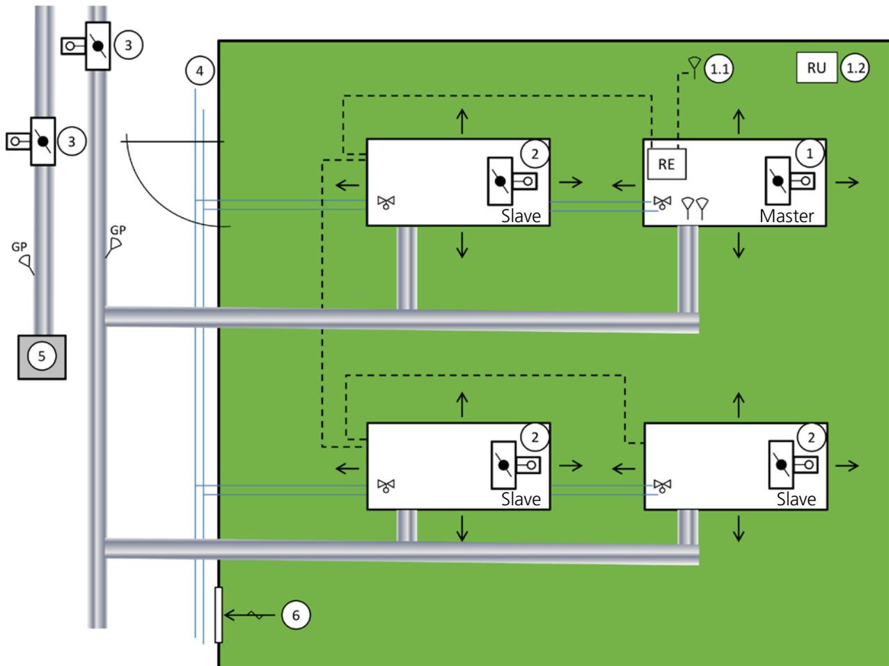
Figure 15. Typical room 1 shows Parasol VAV master with 3 Parasol VAV slaves in an office. Extract air via the air transfer grille (balance on zone level).
