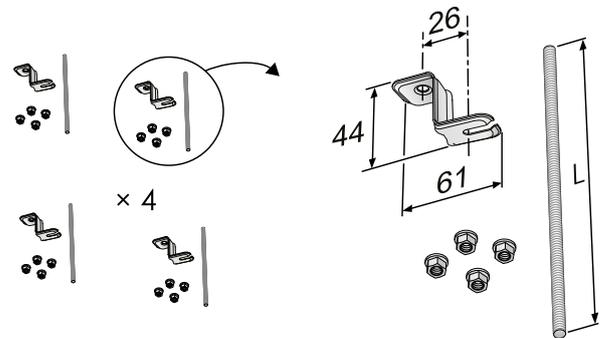
Figure 21. Assembly piece SYST MS M8-1, ceiling mount and threaded rod
