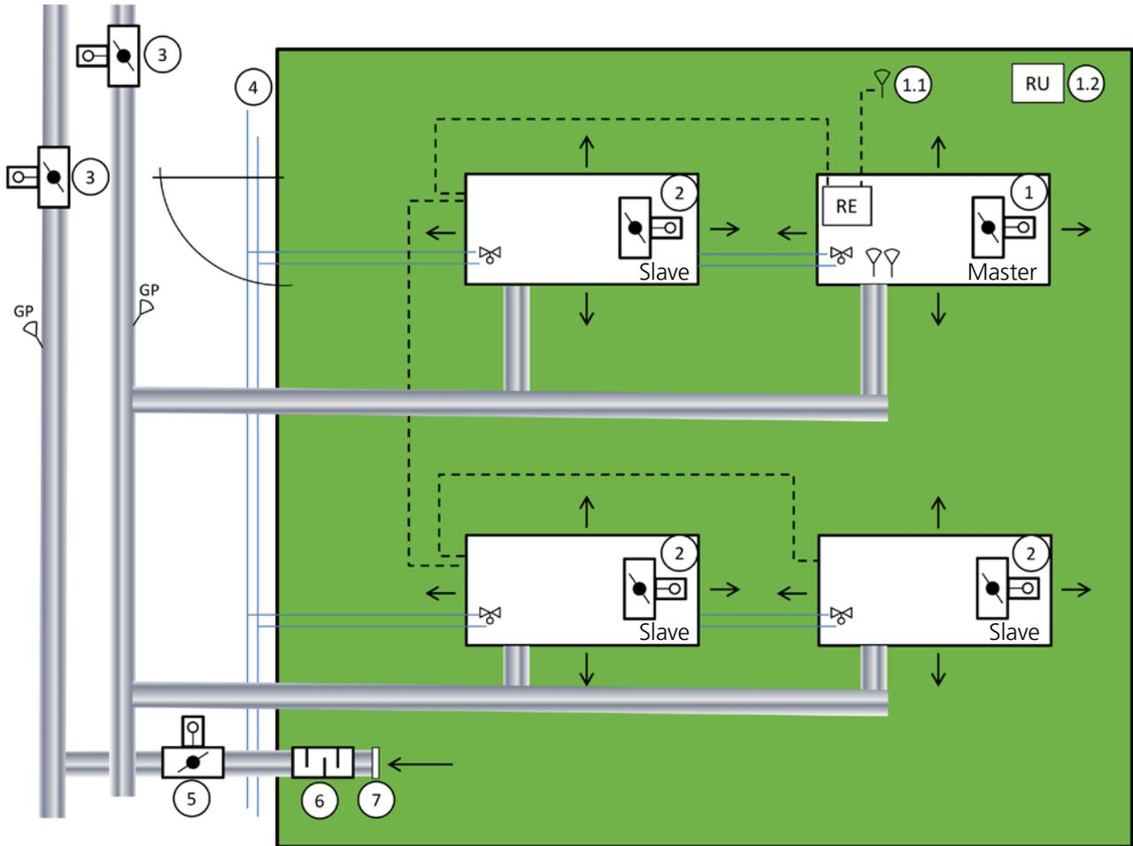
Figure 16. Typical room 2 shows Parasol VAV master with 3 Parasol VAV slaves in an office. Supply and extract air in balance.
