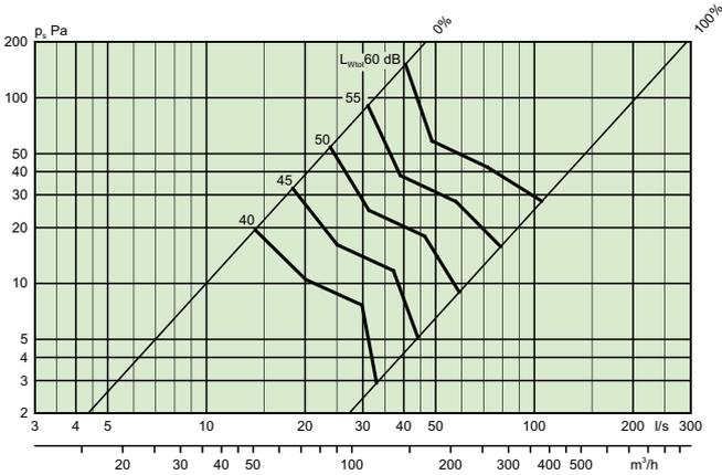
Table 11. Orifice Attenuation  $\Delta L$  (dB) Parasol EX 690
