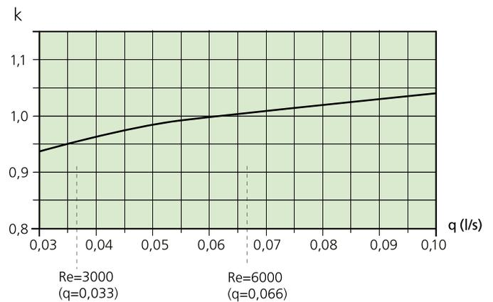
Chart 4. Pressure Drop – Cooling Water Flow
