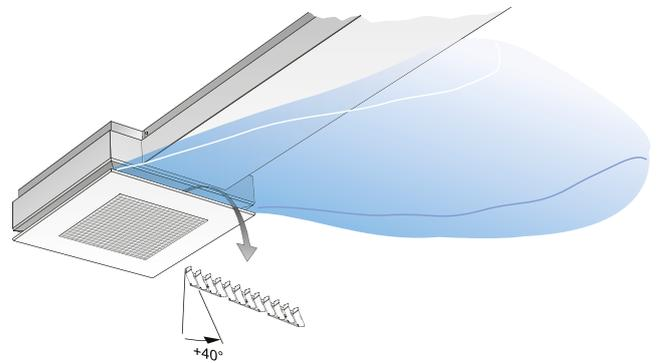
Figure 8. Possible settings for the ADC<sup>II</sup>, X-shape
