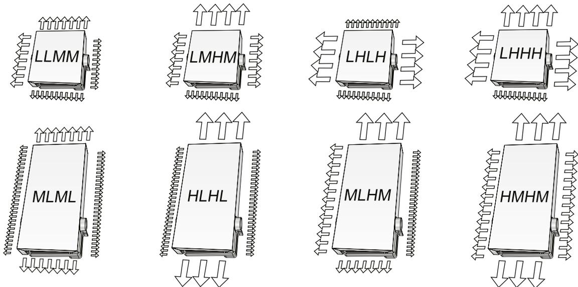
Figure 21. Examples of optimized nozzle setting.
