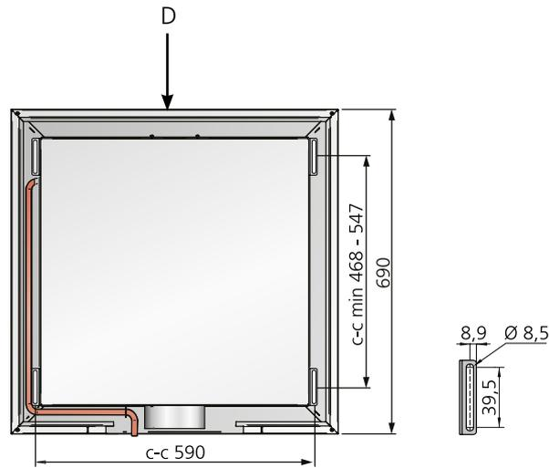
Figure 23. Parasol EX 690 top view with connection bracket
