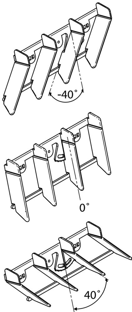
Figure 6. ADC<sup>II</sup>, setting range from -40° to +40° in increments of 10°
