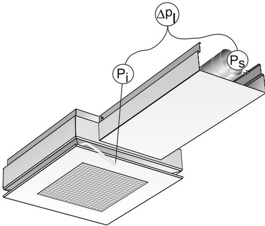
Figure 22. Pressure Conditions - Air
