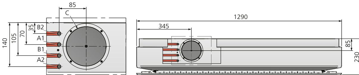
Figure 26. Parasol EX 1290, top view with connections
