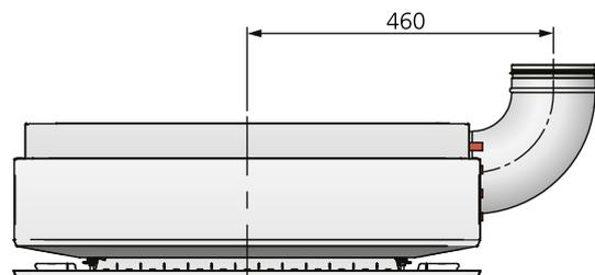
Figure 28. Connection with duct bend, end view
