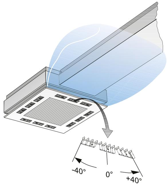
Figure 7. Possible settings for the ADC<sup>II</sup>, Fan shape
