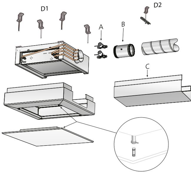
Figure 17. Diagrammatic sketch for suspending the Parasol EX and housing
