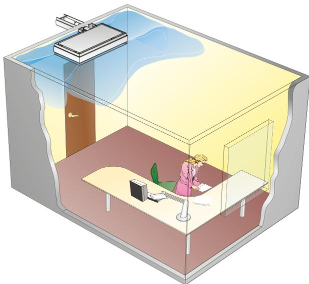
Figure 9. Parasol EX as a rear edge solution
