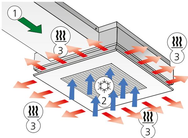
Figure 3. Variant B: Heating function (also includes cooling function)
