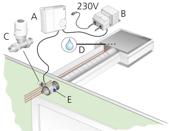
Figure 15. Installation with valve, actuator and damper in corridor
