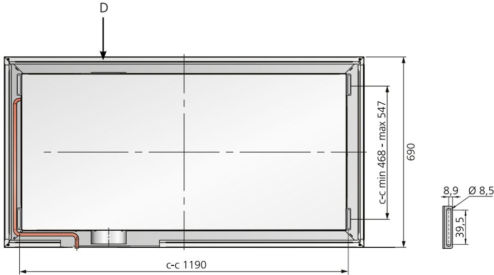
Figure 25. Parasol EX 1290 top view with connection bracket
