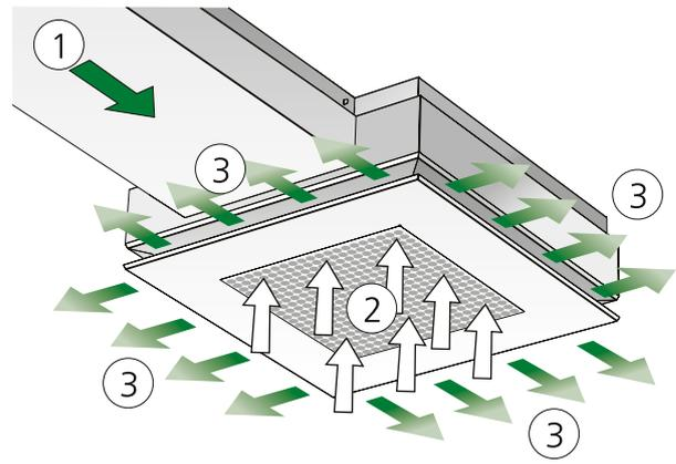
Figure 4. Variant C: Supply air function
