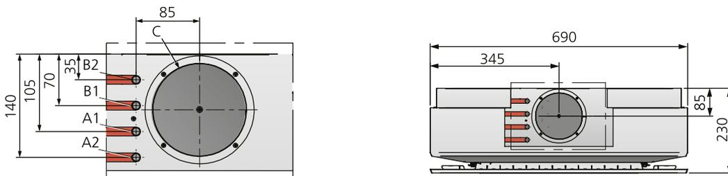
Figure 24. Parasol EX 690, top view with connections
