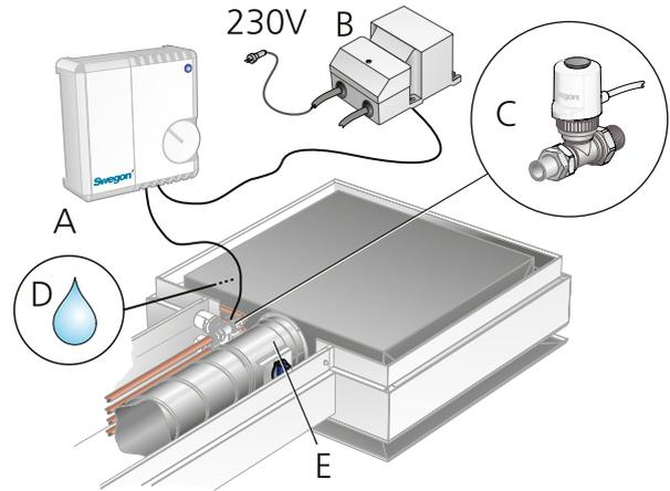
Figure 14. Installation with all components in the room
