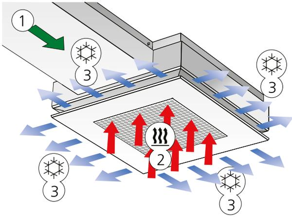
Figure 2. Variant A: Cooling function
