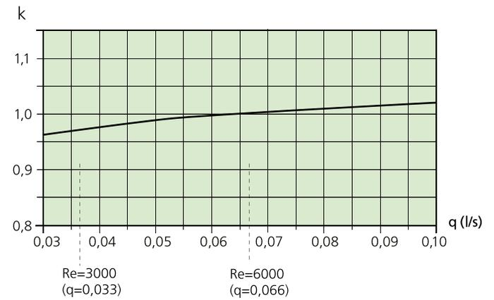
Chart 3. Corrected Capacity – Water Flow, Parasol EX 1290
