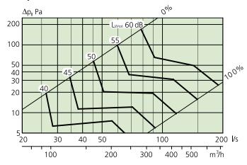
Diagram 3 shows the total generated sound power (L  $_{\rm Wtot}$  dB), as a function of the air flow and pressure drop across the damper. By correcting L $_{\rm Wtot}$  with the correction factors from Table 14, the sound power level for each octave band (L $_{\rm W}$  = L $_{\rm wtot}$  + K $_{\rm ok}$ ) can be obtained.
