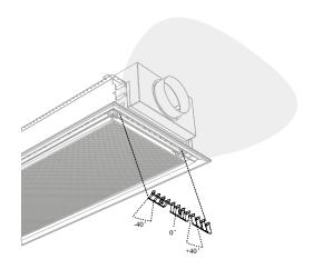
Figure 6. Possible settings for the ADC, Fan-shape
