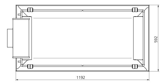
Figure 35. Dimensional drawing, view from above. Air connection on the short side - pos 1.
