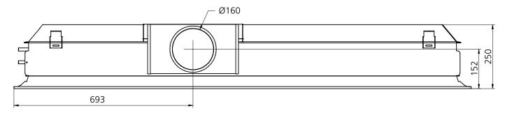
Figure 39. Dimensional drawing, side view. Air connection on the long side - pos 2.
