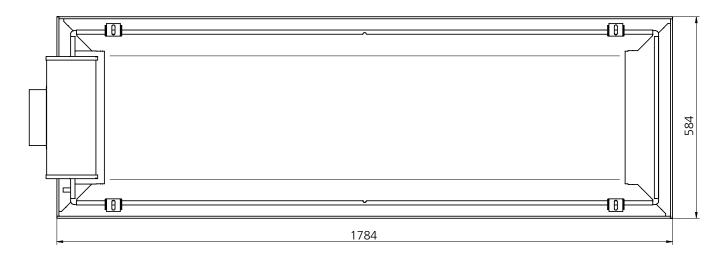
Figure 41. Dimensional drawing, view from above. Air connection on the short side - pos 1.
