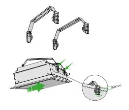
Figure 27. Suspension with quick brackets, PARASOL Z QUICK SUSPENSION KIT
