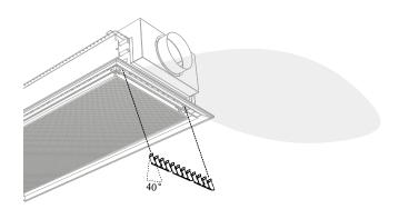
Figure 7. Possible settings for the ADC, X-shape
