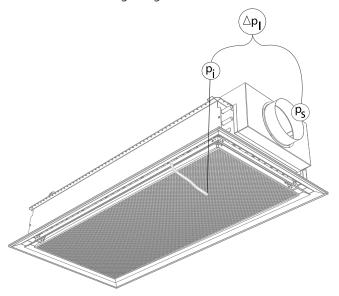
Figure 30. Pressure Conditions - Air
