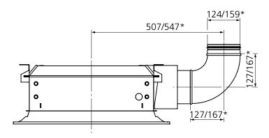
Figure 45. Dimensional drawing, long side connection with bend  $\emptyset$ 125/160 \*=  $\emptyset$ 160
