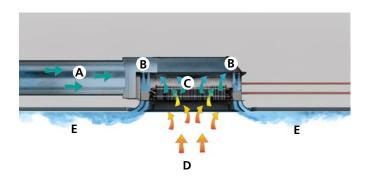
Figure 4. Induction principle in Parasol Zenith
