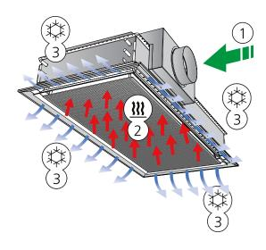
Figure 2. Variant A: Cooling and supply air function
