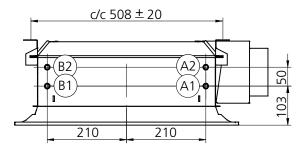
Figure 31. Dimensional drawing, end-view with water connections.
