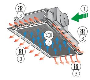
Figure 3. Variant B: Heating and supply air function (Heating only 1200 module and also including cooling function)
