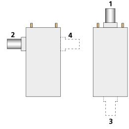
Figure 23. Alternative air connections
