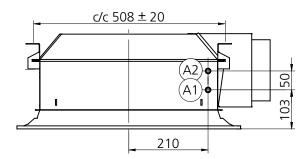
Figure 37. Dimensional drawing, end-view with water connections. Air connection on the long side - pos 2.
