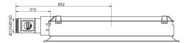
Figure 44. Dimensional drawing, short side connection with the commissioning damper fitted SYST CRPc 9-125/160
