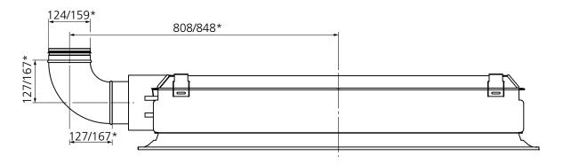
Figure 46. Dimensional drawing, short side connection with bend Ø125/160 \*= Ø160
