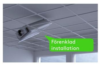
Figure 17. Installation in existing T-bar system
