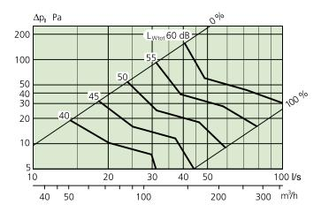
Diagram 2 shows the total generated sound power (L  $_{\rm Wtot}$  dB), as a function of the air flow and pressure drop across the damper. By correcting L $_{\rm Wtot}$  with the correction factors from Table 13, the sound power level for each octave band (L $_{\rm W}$  = L $_{\rm wtot}$  + K $_{\rm ok}$ ) can be obtained.
