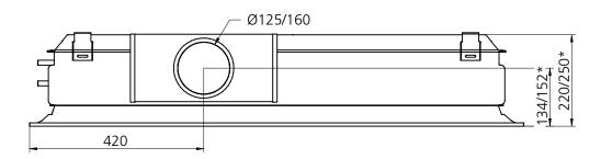
Figure 33. Dimensional drawing, side view. Air connection on the long side - pos 2.
