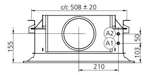
Figure 40. Dimensional drawing, end-view with water connections. Air connection on the short side - pos 1.
