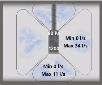
Figure 11. Adjustable air flow per side - 1200 size at 80 Pa total pressure.
