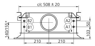
Figure 34. Dimensional drawing, end-view with water connections.
