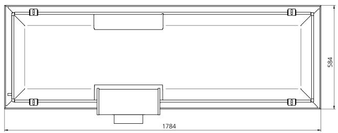
Figure 38. Dimensional drawing, view from above. Air connection on the long side - pos 2.
