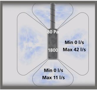
Figure 12. Adjustable air flow per side - 1800 size at 80 Pa total pressure.
