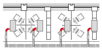
Figure 20. Installation example. Straight air connection, alternative with 90° bend.
