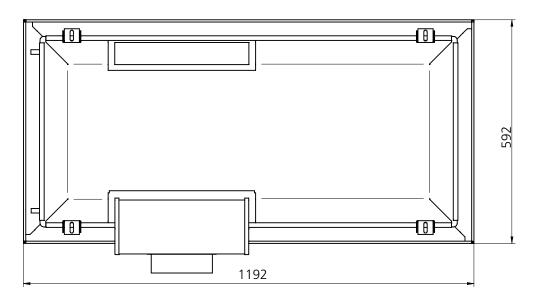
Figure 32. Dimensional drawing, view from above. Air connection on the long side - pos 2.
