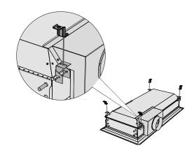
Figure 26. Suspension in four brackets with SYST MS M8
