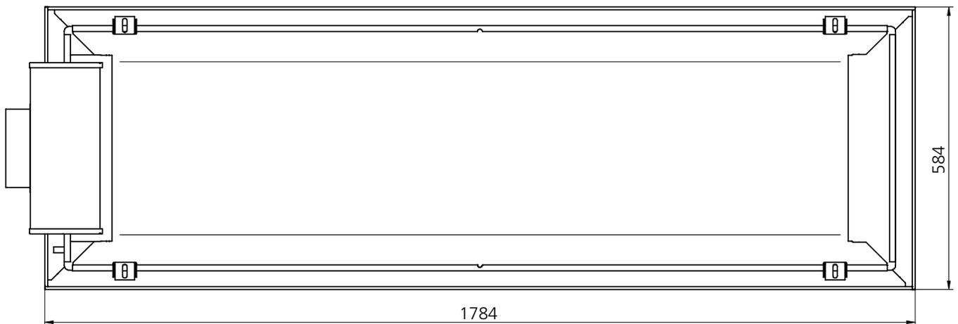
Figure 41. Dimensional drawing, view from above. Air connection on the short side - pos 1.
