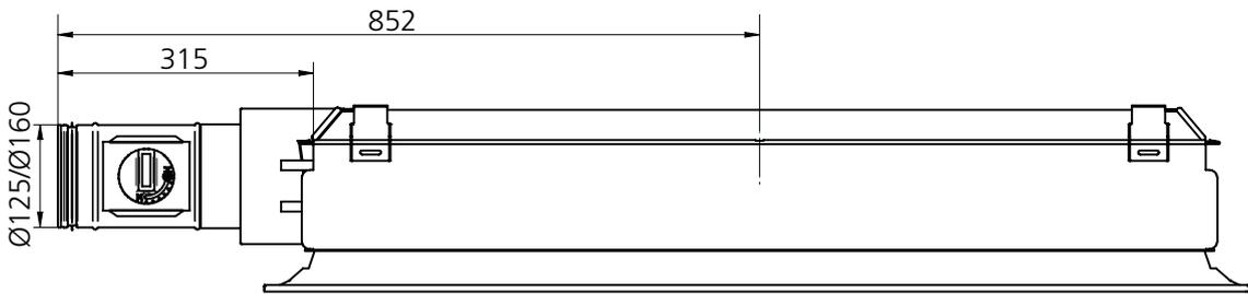
Figure 44. Dimensional drawing, short side connection with the commissioning damper fitted SYST CRPc 9-125/160
