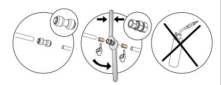
Note that clamp ring couplings require support sleeves inside the pipes.
