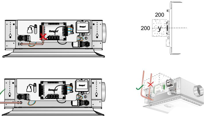
☞ Note the need for a empty space in front of the controller in order to facilitate service.
