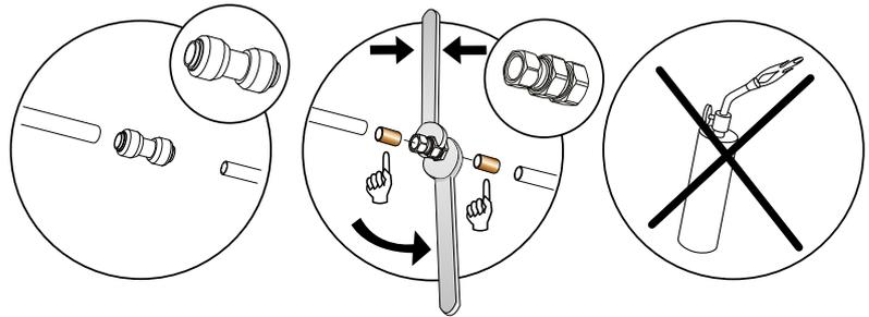
☞ Note that clamp ring couplings require support sleeves inside the pipes.
