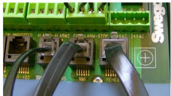
Fig. 8 To connect the cable of the hand-held terminal
