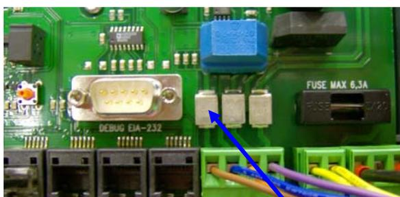
Fig. 3 Thermal fuse for 18 V AC
