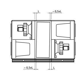
The illustration shows the factory-preset rotor inclination for Fan Arrangement 1. The inclination must always be toward the filter, which means that the inclination for Fan Arrangement 2 is in the other direction.
