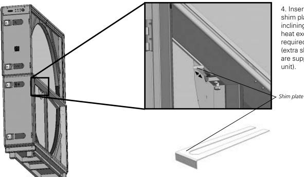
4. Insert or remove shim plates for inclining the rotary heat exchanger to the required inclination (extra shim plates are supplied with the unit).
