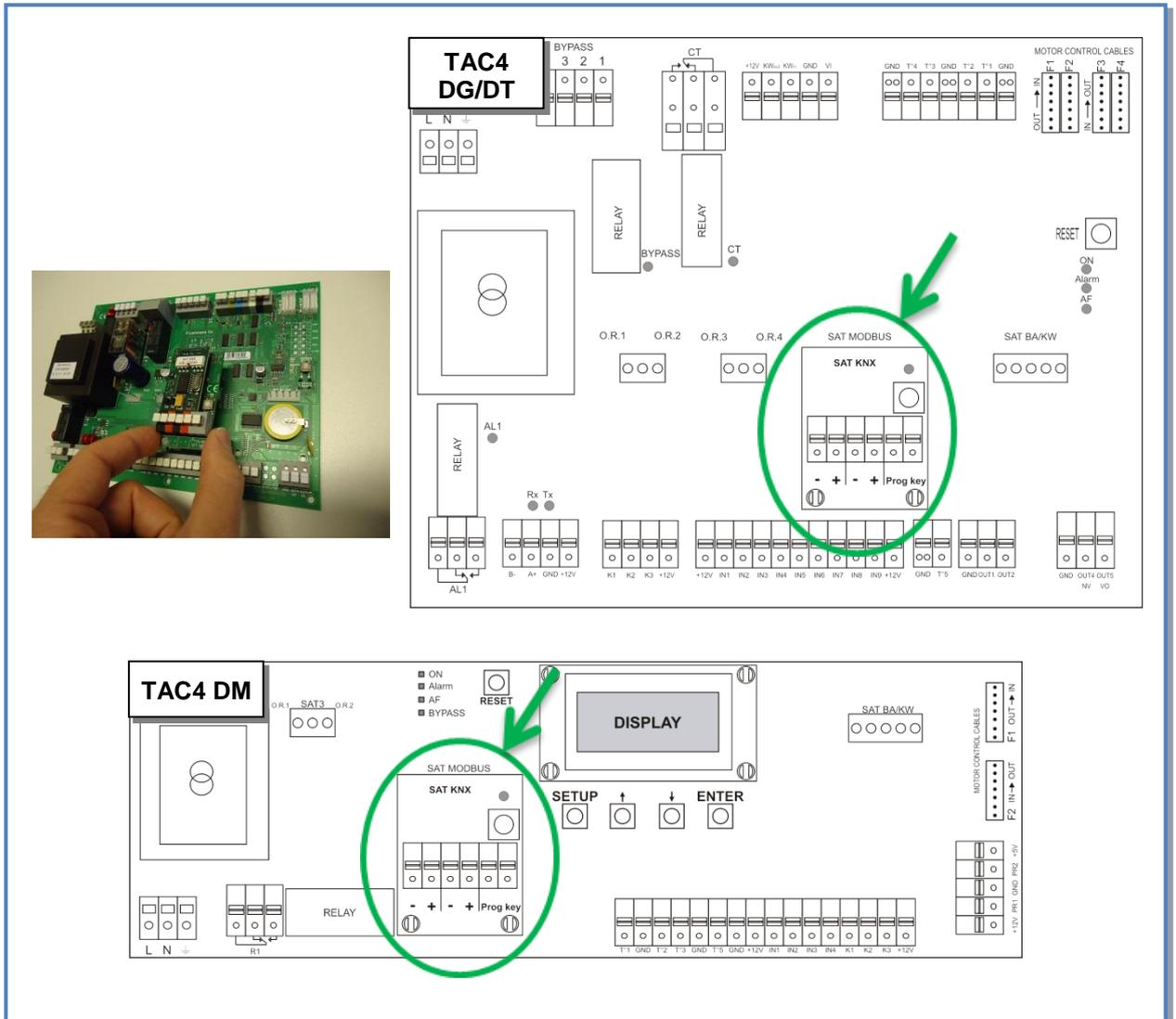
Figure 4 - Plugging of SAT KNX on the TAC4 control board
