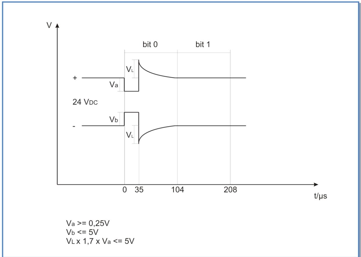
Figure 8 – KNX binary signals shape
