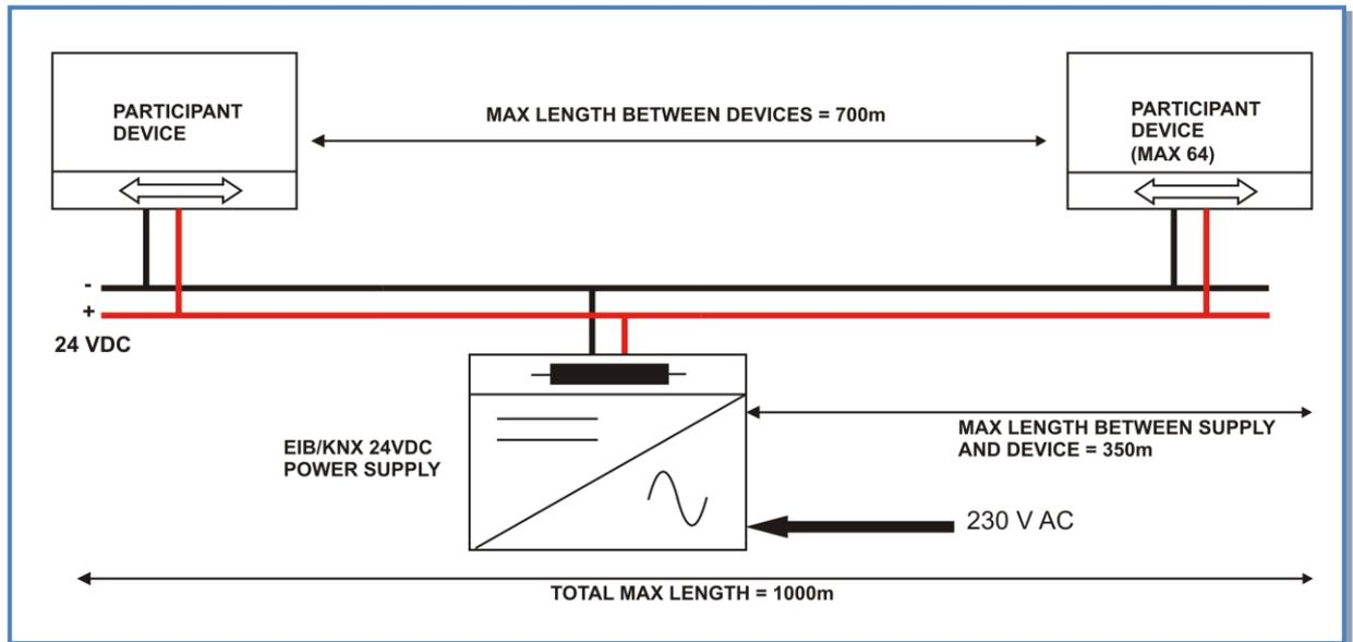
Figure 9 – maximum dimensions in KNX network
