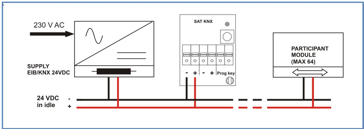
Figure 5 – Wiring to the KNX Network
