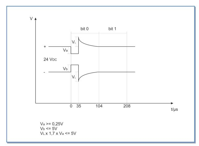
Figure 8 – KNX binary signals shape
