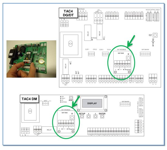
Figure 4 - Plugging of SAT KNX on the TAC4 control board
