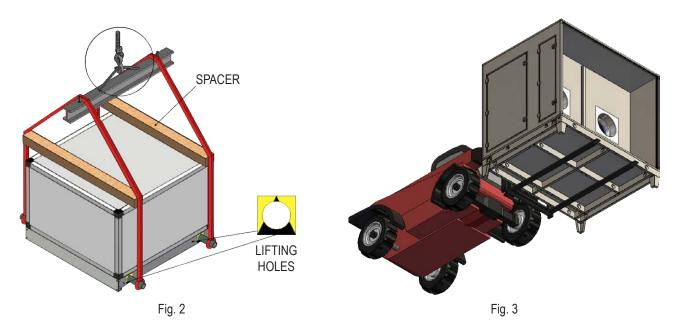
Unit sections should be handled separately, before any assembly or coupling is made. After sections are assembled, it is NOT possible to move the whole resulting unit.
