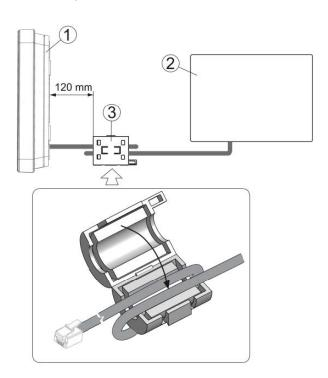
Installation EMC filter: 1 - control panel, 2 - controller module, 3 - EMC filter (type ZCAT1518-073).
