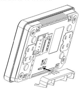
The control panel has built-in magnets, which allows it to be attached without screws to a flat metal mounting surface.
