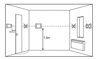
To reduce measurement disturbances avoid locations exposed to strong sunlight, with poor air circulation, near heating equipment, and directly at the door and windows (typically 0.2 m from the edge of the door).
