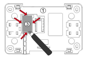
Drill holes in the wall and use screws (max. Ø 3 mm) to fix the mounting frame in the chosen place of the wall, maintaining its proper position (UP). Then attach the control panel to the mounting frame using latches.
