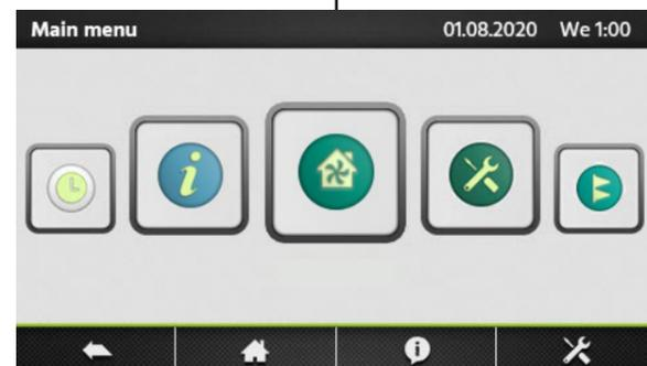
Main menu. See Section 2.1.2. The main menu is presented as a rotary menu. After pressing the "menu"-button at the bottom left corner of the Home Screen, the rotary menu will be shown.
